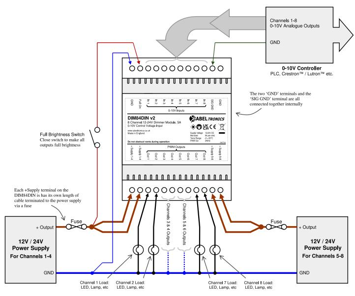
Both power supply GND terminals are connected together
