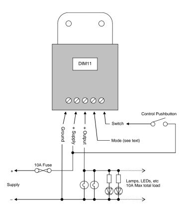
With the Mode input connected to the +Supply terminal, when the lamp is turned on, the previously stored brightness level is retrieved. The level can then be adjusted with a sustained press of the control switch. When the lamp is turned off, or when power to the module is lost, the current brightness setting is stored for retrieval next time.
