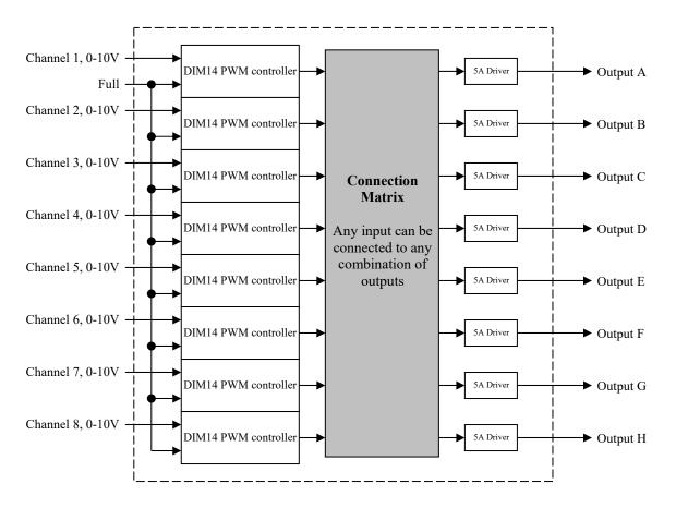
The diagram below shows the dimmer configured as a single channel unit. One channel controls all eight outputs. This configuration permits 40A of total load to be driven from one channel in eight banks of 5A.
