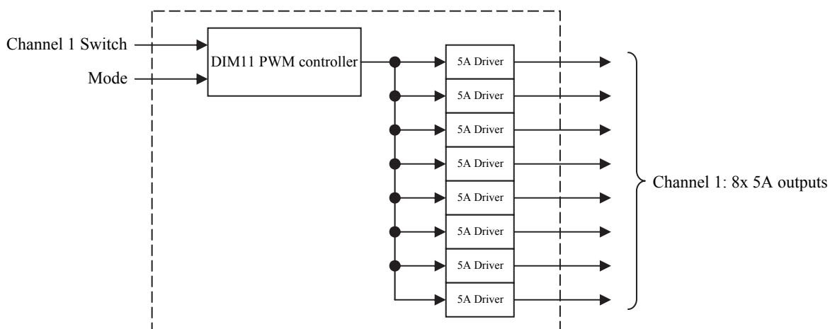
This diagram shows the dimmer configured as a two channel unit. Channel 1 controls outputs A to D and channel 2 controls outputs E to H. Channels 1 and 2 have a total rating of 20A each, with the load split into four 5A banks, per channel.
